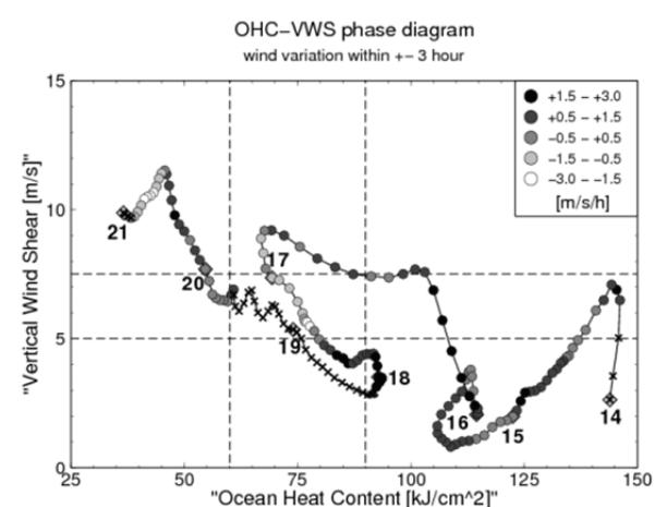
**Fig. 9 :** The PEH diagram using the CReSS-NHOES simulation on T1013. Horizontal and vertical axes show OHC and VWS, respectively. Intensification rate of the TC is calculated by 3 hours before and after the time. Dark and light gray marks show the intensification and decaying at the time, respectively. Crosses show the period when T1013 landfall on Luzon Island.
