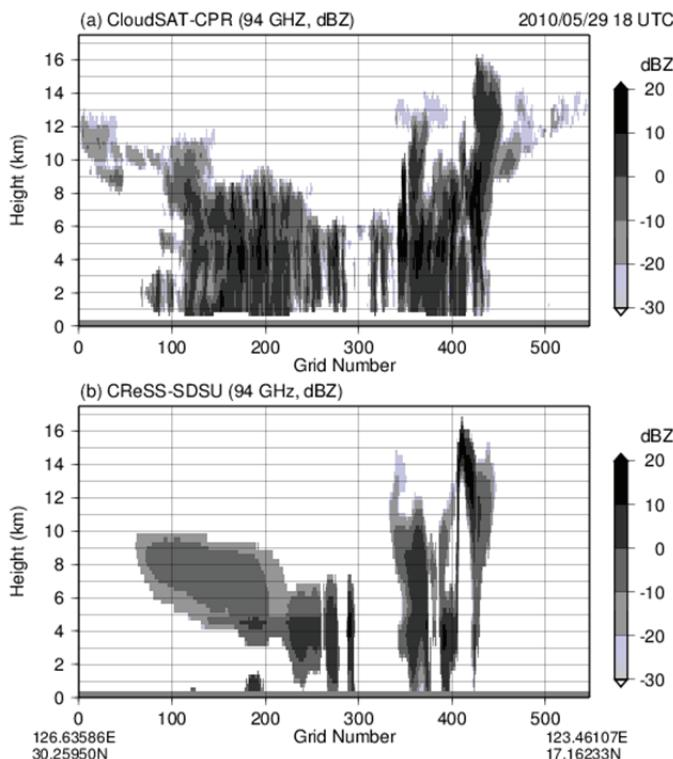
**Fig. 1:** Vertical cross section of (a) observed reflectivity for 94 GHz obtained by CloudSat-CPR and (b) simulated one (CReSS-SDSU) over the Taiwan-Okinawa region at 18 UTC on May 29, 2010.
