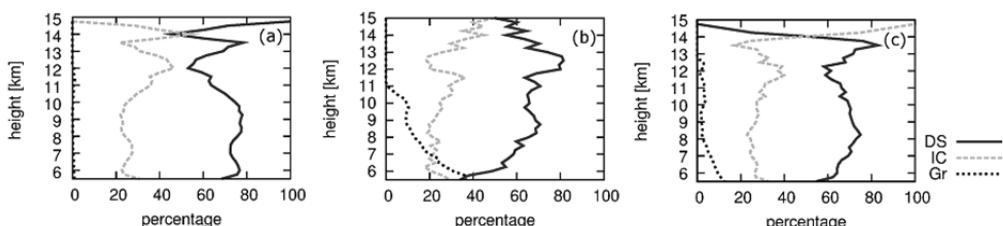
**Fig. 4 :** Vertical distributions of frequency of solid particles; ice crystal (gray broken line), dry snow (solid line), and dry graupel (dotted line) above a height of 5.5 km (around the melting level) for 3 types of the precipitation system: (a) a stratiform precipitation system, (b) an isolated convection, and (c) convective cells embedded in a stratiform precipitation system.
