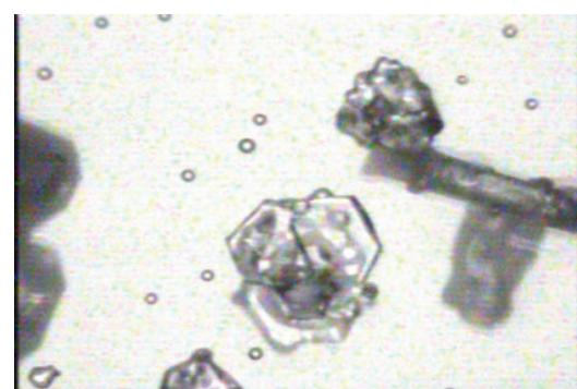
**Fig. 7 :** A particle image obtained by a HYVIS at a height of 6.1 km (temperature -5.2 Celsius degree) launched at 1445 LST from the Aimeliik Site, Republic of Palau. Horizontal and vertical scales of the image are 1.2 mm and 0.9 mm, respectively.
