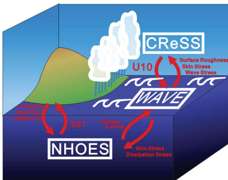
**Fig. 1 :** Schematic representation of the Coupled Atmosphere-Wave-Ocean Non-hydrostatic Model (CReSS-NHOSE).
