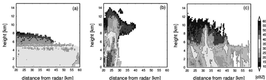
**Fig. 3 :** A sample of RHI images of reflectivity for 3 types of the precipitation system: (a) a stratiform precipitation system, (b) an isolated convection, and (c) convective cells embedded in a stratiform precipitation system.
