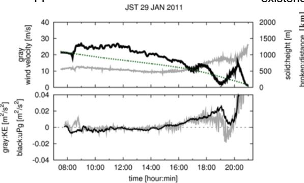
**Fig. 11 :** Time series of the back trajectory analysis starting at 2100 JST on January 29, 2011 calculated using the simulation result. The upper panel shows time series of wind speed (gray solid line), height (solid line), and distance from the starting position of the back trajectory (dotted line) of the air parcel. The lower panel shows time series of kinetic energy (gray solid line) and pressure gradient force (solid line) of the air parcel.
