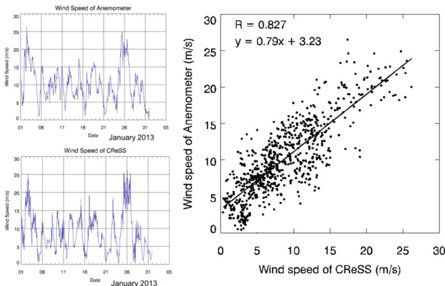
**Fig. 1 :** Comparison of wind speed of anemometer at the height of 50 m on a wind tower in Hegura-jima and CReSS simulation of 2 km x 2 km horizontal resolution for the anemometer point: time variation of wind speed for January 2013 of anemometer (left top panel) and that of CReSS simulation (left bottom panel), and scatter plot of them (right panel).
