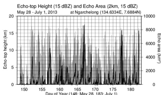
**Fig. 6 :** Time series of echo-top height (gray bar graph) and echo area at a height of 2 km (solid line) from May 28 (DOY = 148) to July 1 (DOY = 182), 2013. Both echo-top height and echo area are defined by 15 dBZ.
