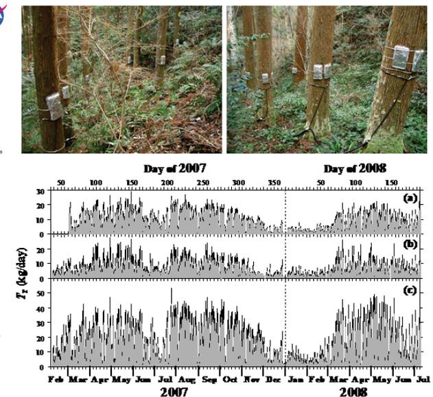
Measurements of individual tree water use (upper panels) and the results obtained on each day at the center of the south-facing slope (a), an upper position (b) and a lower position (c) of the north-facing slope. Using many such sensors distributed over a forest watershed, we can examine the environmental response of forest water use at a catchment scale.
