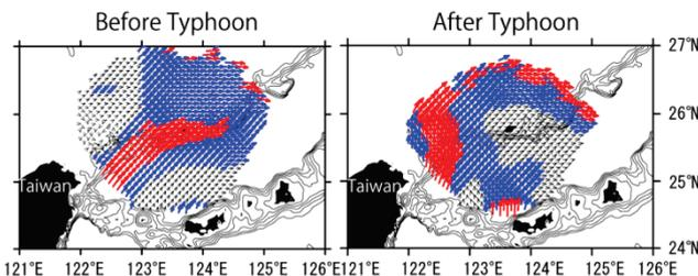
The Kuroshio northeast of Taiwan observed by long-range ocean radar before and after the typhoon passage. Red indicates a current velocity greater than 1 m/s. The Kuroshio flows northeastward before the typhoon approaches and flows northward after the typhoon passage.
