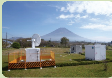
Cloud and precipitation observation near Mt. Fuji using polarimetric and Ka-band radars.
