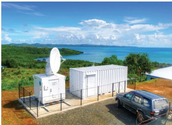
An X-band polarimetric Doppler radar of Nagoya University is installed at Ngarchelong State, Republic of Palau. An intensive observation is conducted in June 2013 to clarify mesoscale convective systems with vortices forming a typhoon over the western Pacific Ocean.
