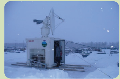
Snowfall observation in Rikubetu-town, the eastern Hokkaido using polarimetric radar.
