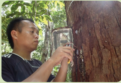
Installation of the sap flow sensor, which measures the flow rate of water in the stem.
